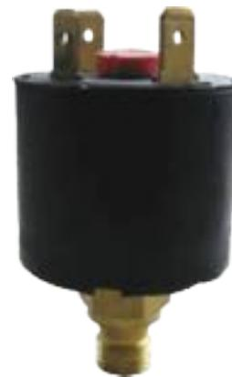
ITA26 is a compact pressure switch capable of sensing pressure range from as low as 0.2 bar up to 6bar and 10 bar. The switching mechanism is an internal snap action switch offering high current capacities with options of SPST, SPDT, normally open and normally closed contacts. It can be widely used in applications, where pressure of air, steam, gas, water etc. need to be controlled accurately and hysteresis is required.
