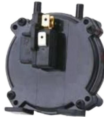
The ITA30 employs a differential pressure to actuate a precision snap switch at chosen pressure setting. This may be the difference between atmospheric and a negative or positive pressure or between any two given pressures. When a change of pressure occurs between the negative pressure chamber and the positive pressure chamber the main diaphragm activates the snap switch at a pre-determined value.
